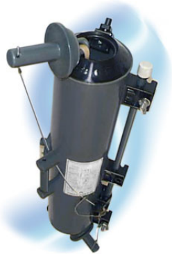
Fig. 2. Niskin Water Sampler and Ponar Grip Submarine Sediment Sampler, and sediments.
