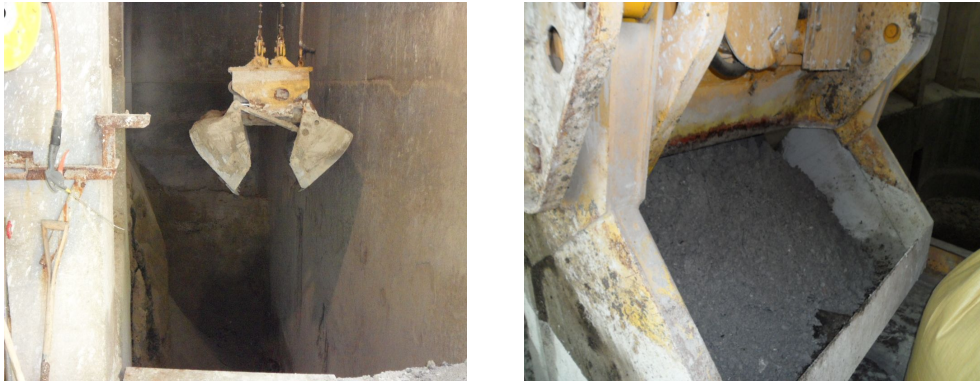
Fig. 5. Bottom ash sampling from ash bunker of incineration plants.
