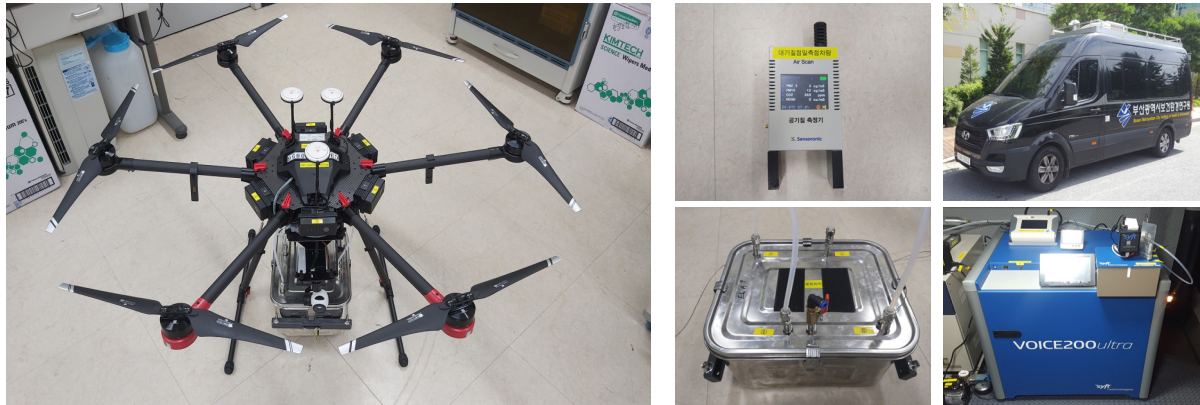
Fig. 2. Drone equipped with an air quality monitoring system.
