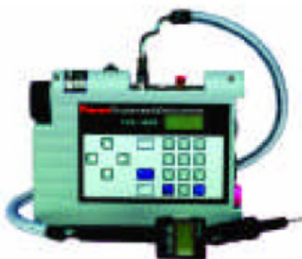
Fig. 1. Figure of potable toxic vapor analyzer (TVA-1000B, Thermo Environmental Instrument, U.S.A)
