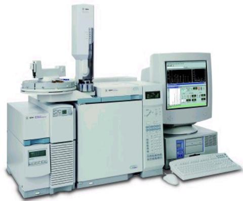
**Fig. 1. Gas chromatograph (Agilent 6890N-5973MSD)**
